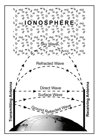
Figure I-1. Propagation Paths for HF Radio Waves
