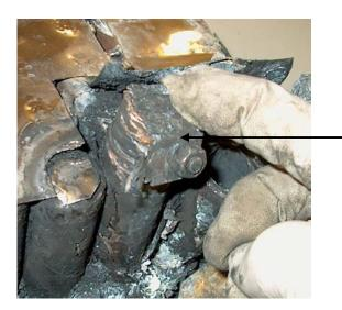
Tab remnant with a portion of the Nickel sheet. This remnant includes the other half of the fuse from Figure 11.
