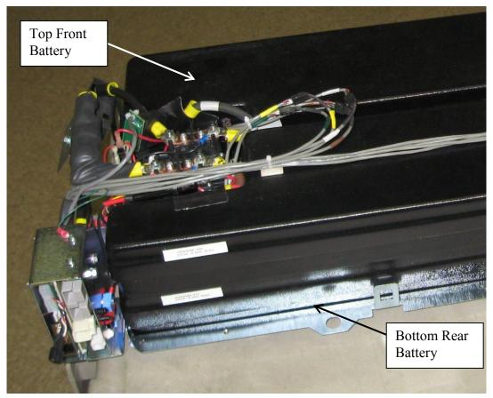
The four batteries are restrained by the top cover which is bolted to the vehicle's chassis in the original battery mounting locations; there is no mechanism for restraining the individual battery assemblies. Figure 6 shows the battery pack with the cover in place.
