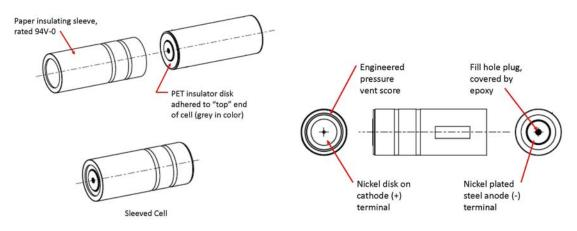
Figure 2--A123 Lithium Ion Cell
