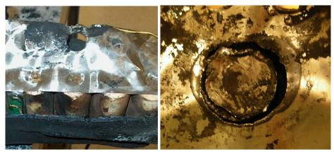
The second feature was located at the Top Front battery on the right-hand side. A cell at the corner of the second series group and located at the corner of a Nickel sheet had become disconnected from the rest of its group, taking the corner of the Nickel sheet with it (Figure 21). The crescent-shaped area on the remaining Nickel sheet shows characteristic signs of excessive heating.
