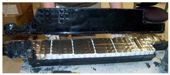
Figure 15--Burn Pattern in a Battery
