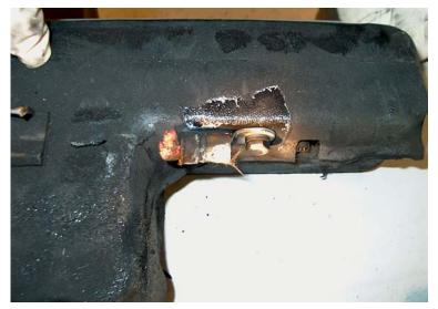
With the clamshell removed, all cells inside that battery could be visualized. It was noted that significant burning was present at the right-hand end, some heat deformation of the plastic and soot on the cells at the left-hand end and little damage in the middle except at the front face where a significant amount of melting occurred (Figure 15).
