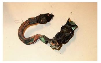
Again, the intact fuse had a severely melted housing but the fuse was still electrically conductive. A microscope examination of the partial fuse shows that the fuse suffered a mechanical break and likely did not melt in an overcurrent condition (Figure 12). Examination of photos taken of the vehicle shortly after the fire show that this fuse was intact after the vehicle was towed to Firmin Ford. The fuse was likely broken during the vehicle investigation in South Carolina.
