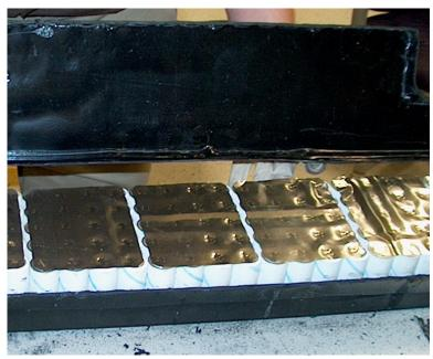
The 600 cells are arranged in four large "batteries" which consist of 160 cells (front batteries, 16 series strings of parallel groupings) or 140 cells (rear batteries, 14 series strings of parallel groupings). These four batteries are created by welding the cells to Nickel sheets (used as bus bars) and then enclosing this construction into a plastic
