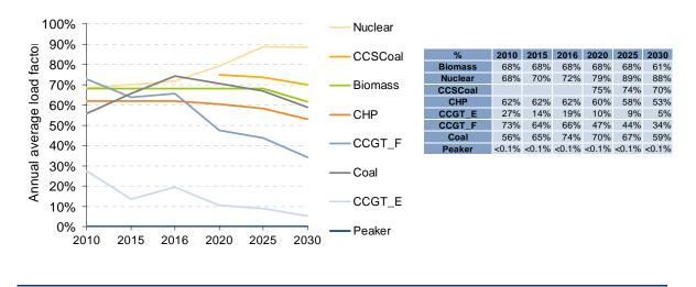
As shown in Figure 68, a similar development occurs in the SEM: load factors of coal plant increase substantially while CCGTs load factors drop to 20% in 2020. New Advanced GT plants perform slightly better than other peaking plants in SEM, but do not exceed a load factor of 5%.
