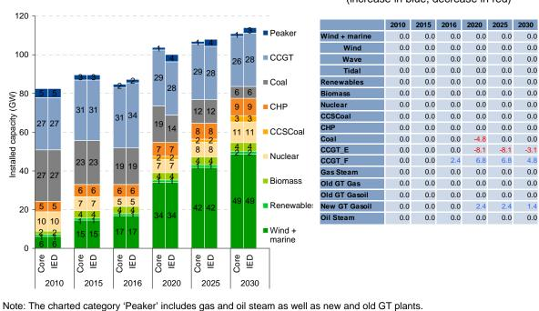
Installed capacity in the IED and Core scenario in GB
