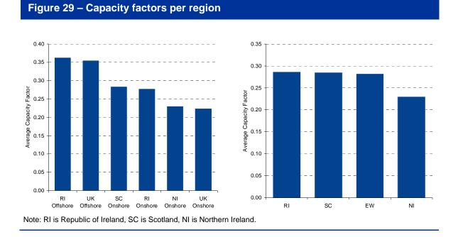
As a rule, it appears that offshore sites exhibit higher capacity factors in general than onshore sites. Due to the large amount of installed capacity offshore, it is to be expected that offshore sites will in effect 'pull up' the average capacity factor for the respective markets. In terms of onshore sites, the Scottish and Rol locations exhibit higher capacity factors in general due to higher average wind speeds, while the wind locations in England and Wales are of lower generation.
