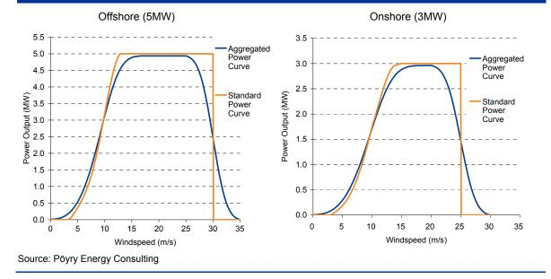
Figure 7 presents the aggregated power curve in relation to the standard power curve for both offshore and onshore turbines. From inspection of Figure 7, the aggregated power curve registers a power output at lower and higher wind speeds than the standard power curve, but the period of peak generation, corresponding to wind speeds of between 14 m/s and 25 m/s (or 30 m/s for the offshore turbine) in the standard power curve, is shorter in the case of the aggregated power curve.
