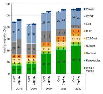
Installed capacity in the Capacity payment and Core scenario
