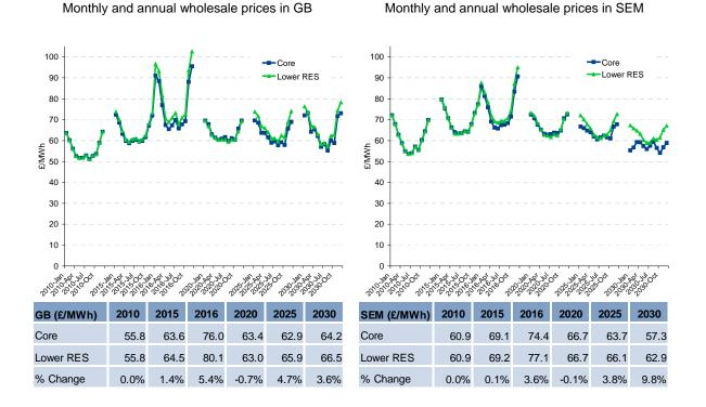
With the assumed installed capacity, the renewable share of generation reaches 26% in the Lower RES scenario rather than 30% in the Core scenario in 2020 in GB, and 40% instead of 51% respectively in 2020 in SEM.
