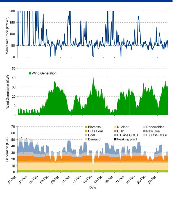
Figure 54 – GB system profile in 2030 based on February 2006
