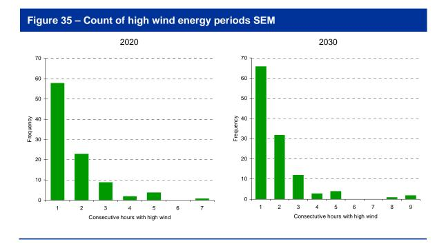
As in the low wind energy case, the distribution of high wind periods is skewed towards shorter duration instances, with the maximum duration being 9 hours in the SEM and 16 hours in GB in 2030, and 7 hours in the SEM and 12 hours in GB in 2020. However, the
