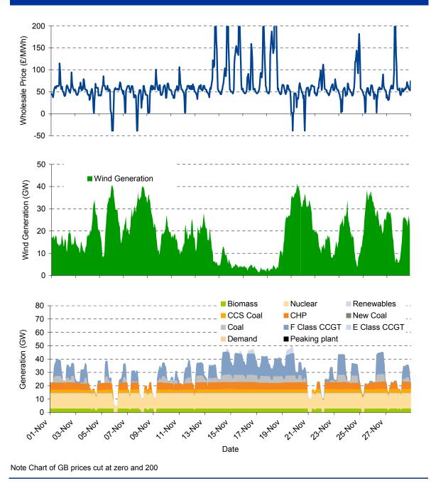
Figure 2 shows how the GB electricity markets reacted during 2030. There are periods of nuclear plant being turned down to permit very high volumes of wind generation – particularly from 21 November. A week earlier, wind generation dropped below 5GW continuously for 4 days which led to a period of very high prices.
