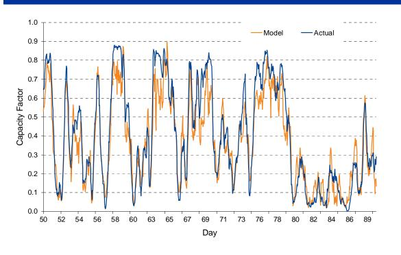
Figure 24 presents the correlation between the wind model data and the EirGrid wind output data, and confirms that the model is in good agreement with the recorded generation data.
