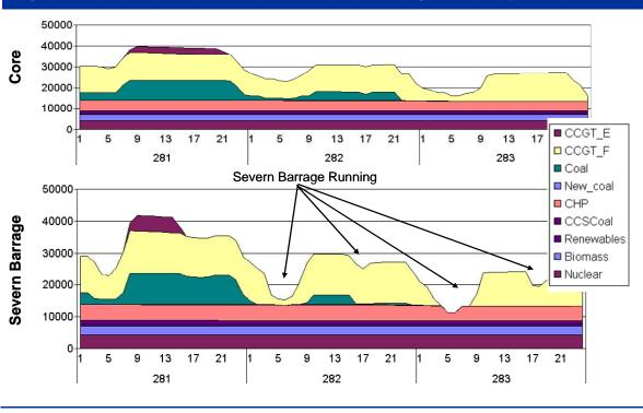
Figure 78 – Plant operation in GB in the Severn barrage sensitivity
