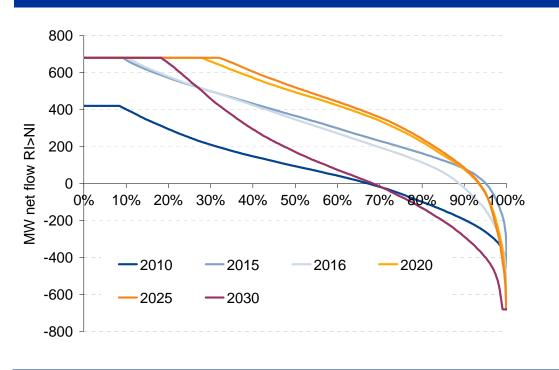
Figure 131 – Net Flows from RI>NI (Duration Curve) in SO Dispatch run
