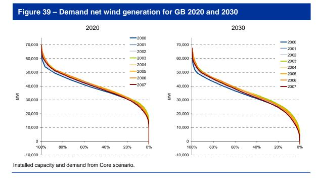
Figure 39 shows the duration curves for demand net wind generation for the GB market in 2020 and 2030. A similar pattern is visible – with variation between Monte Carlo years due to the coincidence of wind and demand. As wind generation increases, the number of periods when there is little demand to be met by thermal generation increases – in 2020, 20% of the time, demand net wind is less than 30GW, whilst in 2030, it rises to 30% of the time.
