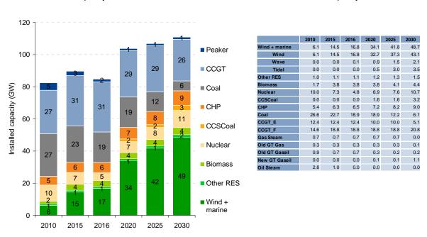
Installed capacity in the Core scenario in GB
