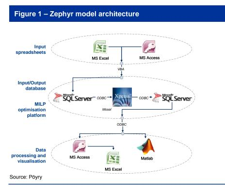
Zephyr is a Mixed Integer Program (MIP) based around Xpress-MP<sup>1</sup> written specifically for this project, which schedules plant by optimising overall variable costs of generation<sup>2</sup>, including start-up and no-load<sup>3</sup> costs across the GB and SEM electricity markets. Optimising start and no-load costs introduce binary<sup>4</sup> variables for whether a plant starts and whether it is on. For thermal plant, Zephyr includes some plant dynamics, including
