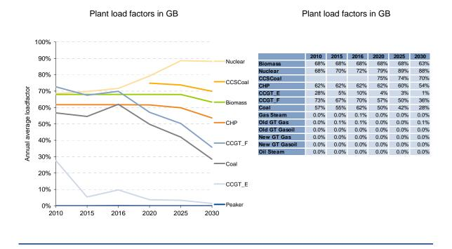
In the SEM, load factors of both coal and CCGT plant are reduced significantly as a result of the higher wind penetration. Load factors of both coal and CCGTs rise in 2016 due to the high prices in GB – exports from GB to SEM drop significantly and load factors in Ireland rise. After 2016, coal load factors keep falling, dropping to under 50% by 2020 and to 35% in 2030, whilst CCGTs have load factors below 20% by 2030.
