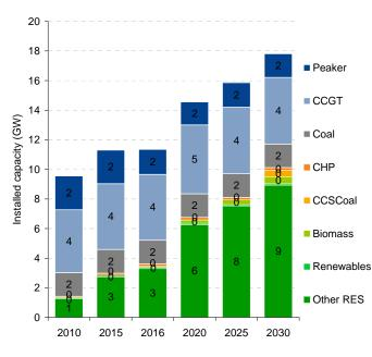
Installed capacity in the Core scenario in the SEM
