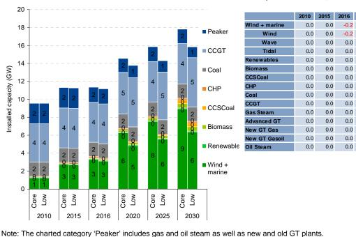
Installed capacity in the Lower RES and Core scenario
