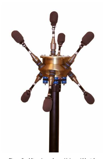
Figure 2 – Microphone Array, Hub, and Mast Assembly
