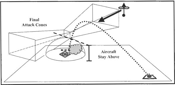
Second, when the aircraft are not laterally offset from the artillery gun target line or mortars are being fired continuous then the aircraft are required to remain above the maximum ordinate of the indirect projectile plus a 1000 ft AGL buffer.
